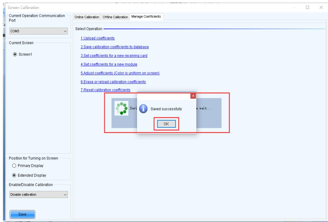
7. After calibration finished, select *Chroma calibration* or *Brightness calibration* and *save* for enable calibration function.
