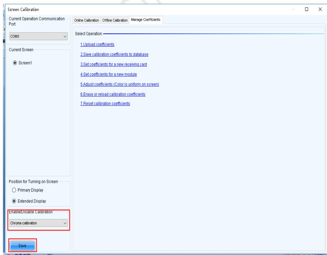
8. After process finished, *saved successfully* notice will appear, select *ok* to end the enable calibration (chroma or brightness) process.
